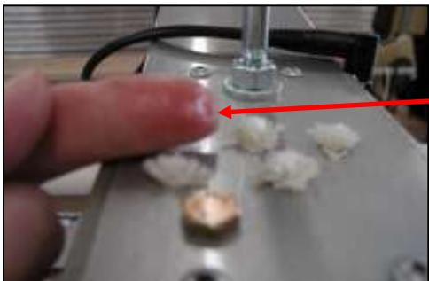
Rub your finger across each of the 5 oiling wicks; it should be wet with oil. If any wick is dry, add one to two drops of oil to that wick.
