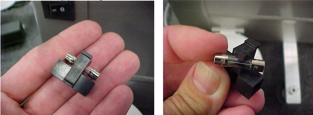
In the event that the fuse would blow, a spare fuse has been packed inside a sliding drawer just behind the active fuse. Using your fingernail or small screwdriver, push on the side of the fuse drawer as shown, and the spare will come out. Use it to replace the burned out fuse.
