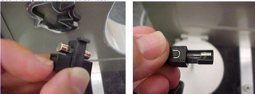
Replacement fuses can be purchased at Radio Shack, or from APQS. Fuses needed for machines are all 250 volt SLOW BLOW fuses – they must be the SLOW BLOW fuses and not the Fast-Acting type usually found in hardware stores. The amperage varies between machines...
