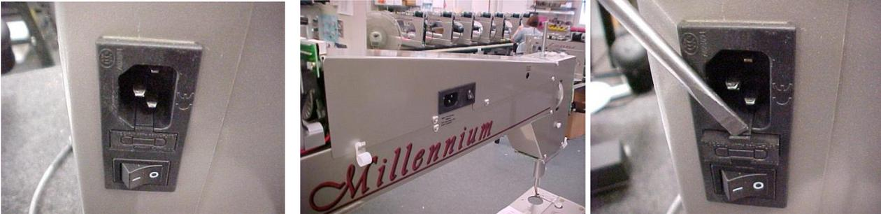
The fuse currently protecting the machine is exposed in the drawer.
